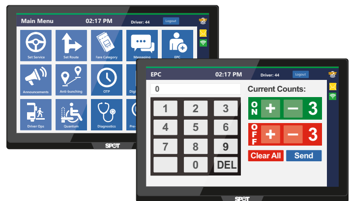
MDT Main Menu (left) and Electronic Passenger Counter module (right).
